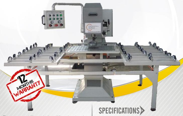
There are two drilling spindles. When the glass is put onto the table, ,it is fixed pneumatically and lower spindle will rise up automatically to drill. Then the upper spindle will drill the top side of the glss and thus, the hole is drilled. The cooling water runs inside the core drill so that the cooling effect is directly acted onto the glass without any loss. Tapping or chamfering can be made on the hole for particularly purpose.
